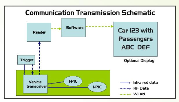
On entering the vehicle, and or at a later time (depending on the business rules), each individual activates their I-PIC. The identification details of each person is captured by the vehicle transceiver. When the vehicle subsequently passes through a 'trigger zone' the details of the vehicle and its passengers are transmitted via a proprietary 2.45 GHz signal to the RFID reader, which in turn communicates to the local server. The reader/server communication can be either ethernet or WiFi.
